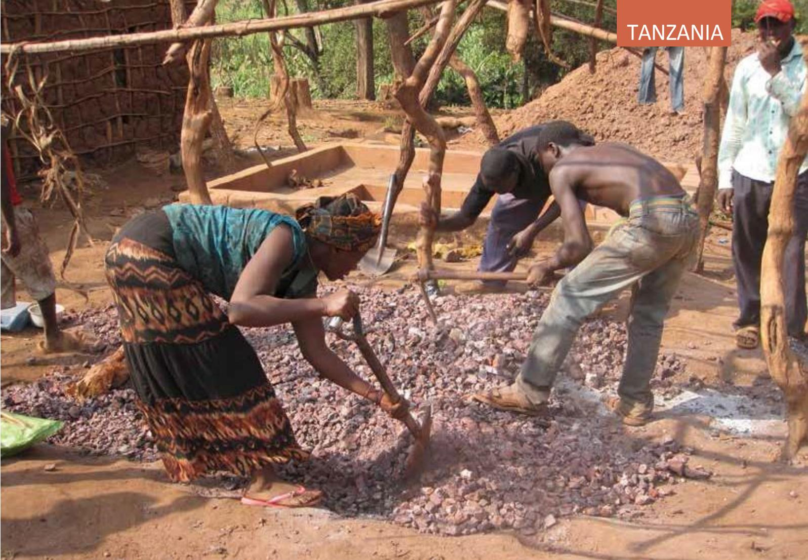
» **GOLD ORE IS CRUSHED** by hand, then processed in a drum and pulverized until it resembles flour. The powder is mixed with mercury and washed in a feed system in which gold is extracted.
